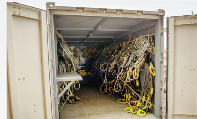
TIGER 8' X 20' DNV 2.7-1 OFFSHORE CONTAINER LOADED WITH SLINGS & RIGGING
